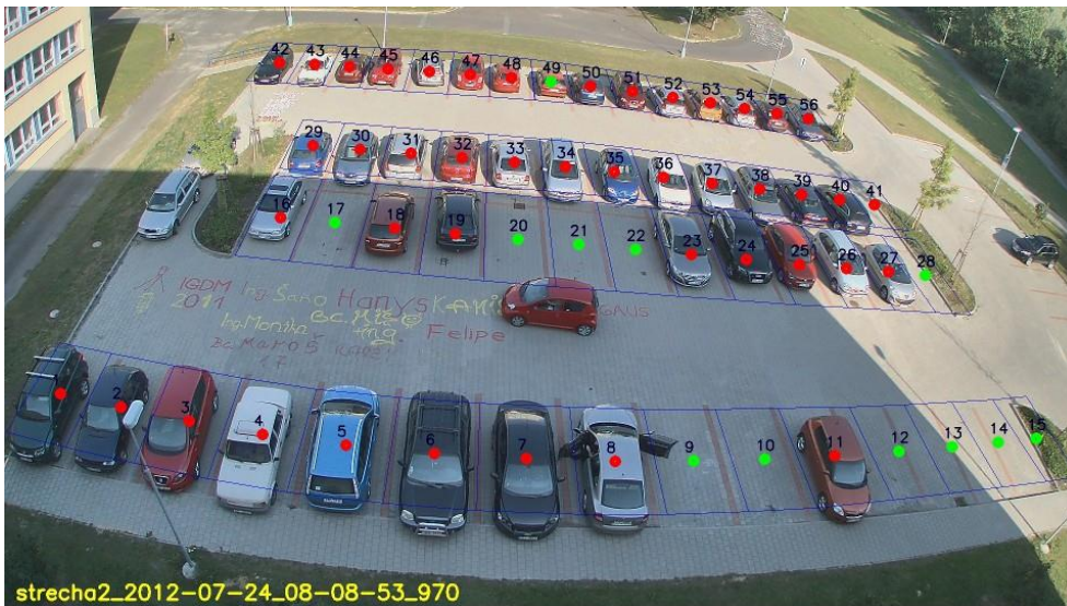
Figure 6.4 Pole mounted technology to determine spaces available in an open air car park
