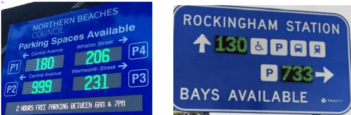
Figure 5.1 Examples of useful variable message signage
