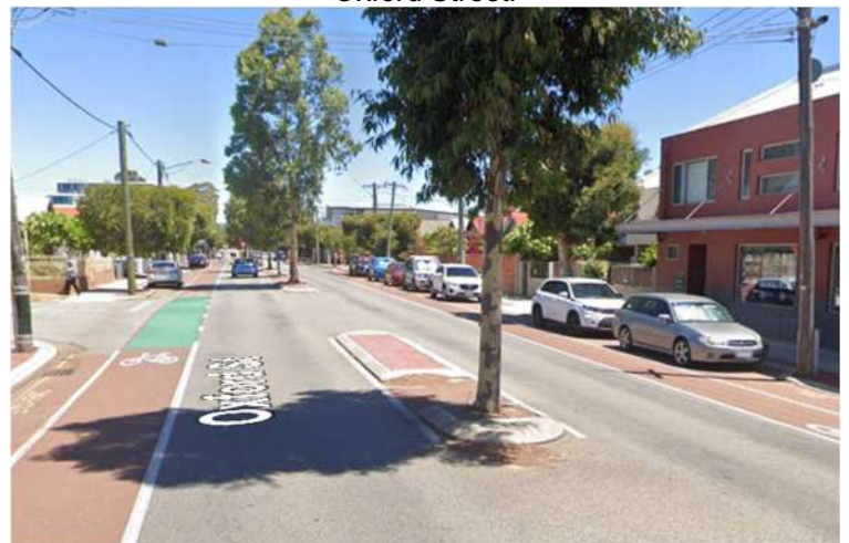
Figure 12 – Oxford Street contains on-street parking, a pedestrian path network and bicycle land.
