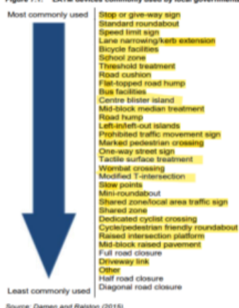
Figure 7.1: LATM devices commonly used by local governments
